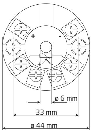
**Mounting of sensor wires**
