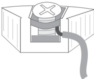
Wires must be mounted between the metal plates.
