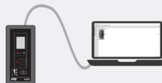
Connection of ConfigMate 4590 to a PC in Docking Mode
