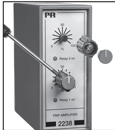
Picture 2: Removal of knobs.
