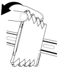
Remove the system 3000 units from the rail by lifting the DIN rail mounting clip.
