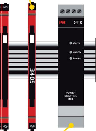
Protective fuse: Located inside the PR 9410.
