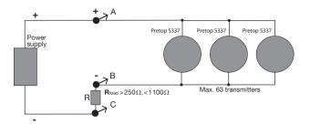
The outputs of max. 63 transmitters can be connected in parallel for a digital HART® 7 communication on 2-wires.
