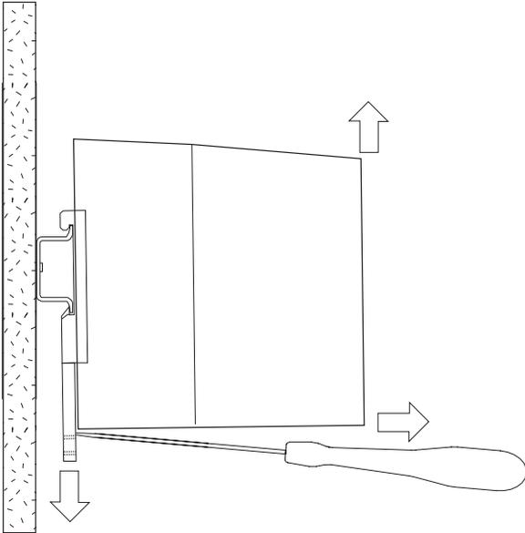
To allow for easy product change the DIN rail mounting clips can be set in the down/release position.
