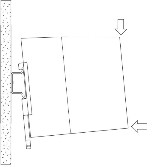
Remove the backplane from the rail by lifting the DIN rail mounting clips:
