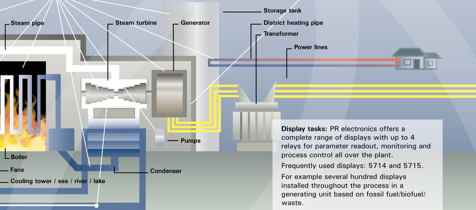
**Display tasks:** PR electronics offers a complete range of displays with up to 4 relays for parameter readout, monitoring and process control all over the plant.
