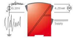
Electrostatic filtration: Electrostatic charges typically occur in the plastics industry. When galvanic isolation is used, PLCs and SCADA systems are protected against breakdown. 4...20 mA
