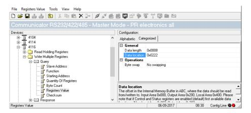
Enter the Anybus data location of the register values that should be written to the node Please note, that there is room for the trigger byte address at 0x0220.
