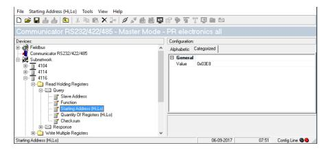
PR electronics 4116 Modbus Manual defines the scaled output value as a double integer on register address 1000 with a register quantity of 2.
