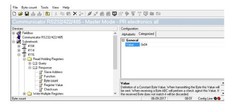
E.g. in "Byte Count" type "4" to prepare Profinet to transfer 4 bytes.
