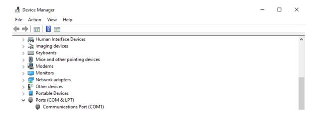
Check your PC's Device Manager for which COM# port the Anybus Communicator is assigned to.
