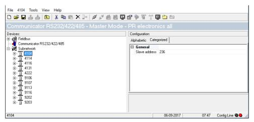
Select a Node, and write the Modbus Address in the "Slave Address" box The "Slave Address" is now automatically set in both the "Query" and the "Response" functions.
