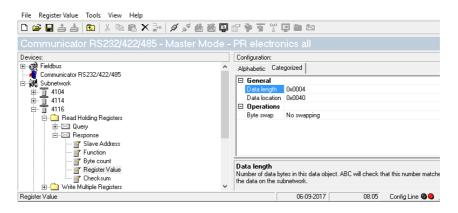
Select the "Register Value", which specifies the receiving input address in the plc. In "Data length" type "0x0004" to specify that a double word will be sent.
