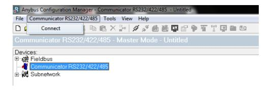
Select the Communicator RS232/422/485 device and press connect.
