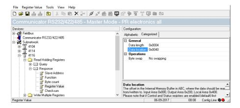
"Data location" specifies where in the Profinet data package this data is located. This means that each register value can be mapped wherever it is convenient. This mapping is not automatic and to begin with, it might help the user to setup this location with a distance of multiples of 0x0010 to be sure that the registers do not overlap/collide.
