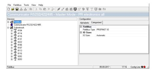
The PR configuration file includes one of each supported modules in the 4000/9000 series. The individual devices/nodes can also be loaded or saved as XML files.
